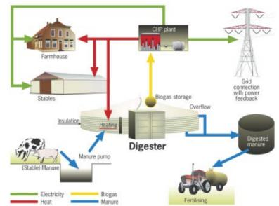
Flow sheet an anearobic digestion system.
