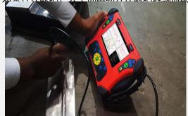
PACE – PDF Field Reports from inspections are instant, showing defect size, length and depth along with the ability to take a photograph to insert into the inspection report.
